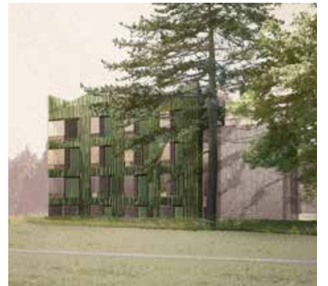
2. The Meadow Building. The Meadow Building is at the centre of the proposals. Ceramic cladding achieves visual variation through a range of depths of fin and criss-cross patterning along with glazes and reflective surfaces.
